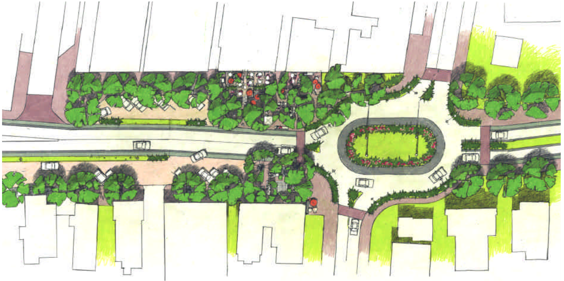
West End illustrative plan with new pedestrian destination and modern roundabout at Sisson Avenue.
